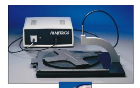
Manually maneuverable wafer chucks make sample handling easy
